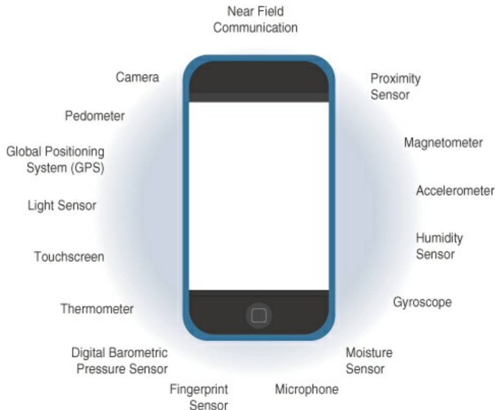
Figure 3-2 Sensors in a Smart Phone
