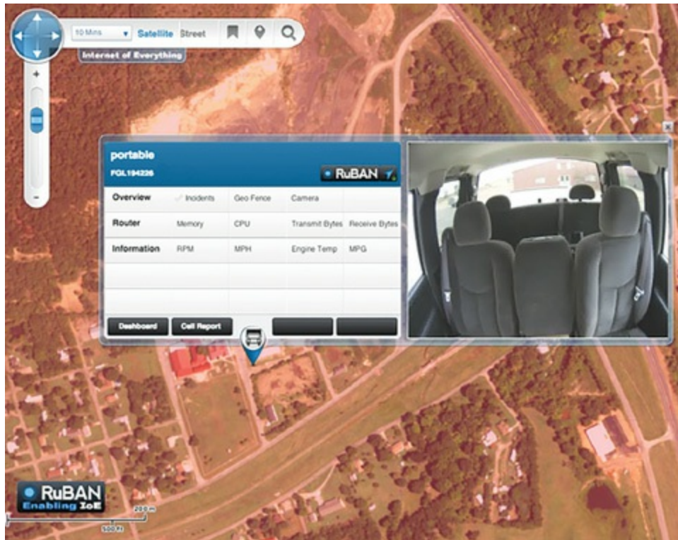
Figure 15-16 Live Viewing of Bus Cameras
