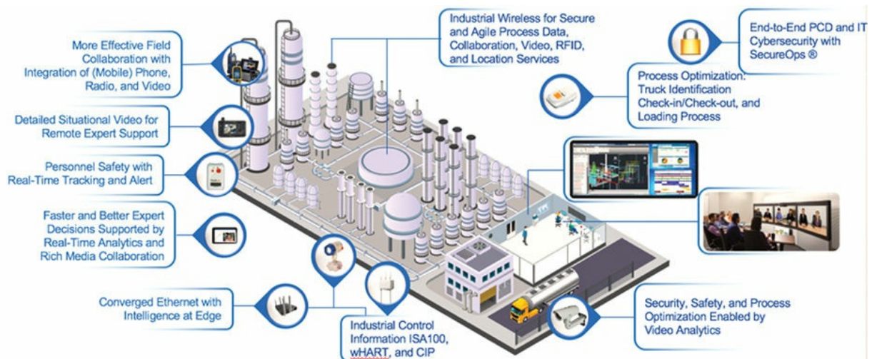
Figure 10-11 Connected Refinery IoT Use Cases
